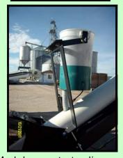
Model mounts to dispense product directly into hopper or conveyor. Can be wired direct to conveyor switch or separate 60' wiring harness.
